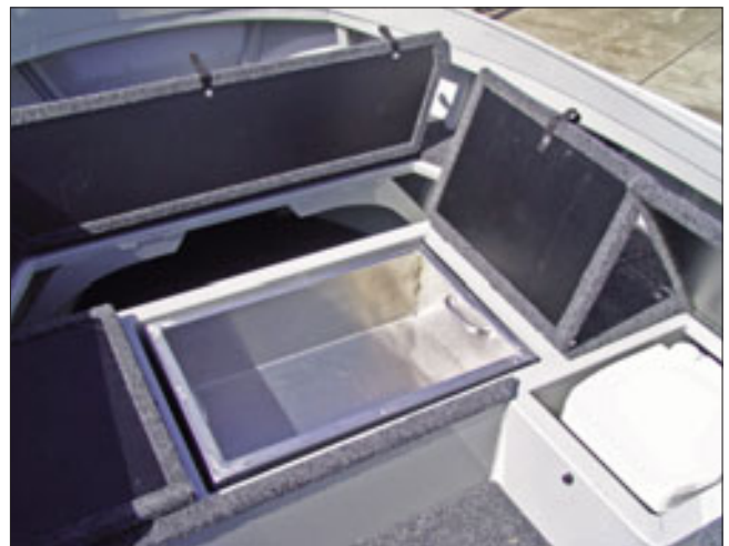
Construction and development shots . . . Makocraft's pressed plate ally construction technique has been tried and proven in thousands of boats over the years. Note the huge lift out fish box, toilet under the casting platform, and (left) the reinforced mounting plates for the electric outboard and the 12v drum anchor winch planned for this rig.
