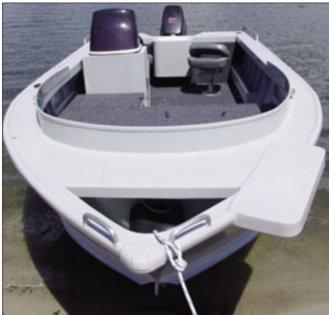
Construction and development shots . . . Makocraft's pressed plate ally construction technique has been tried and proven in thousands of boats over the years. Note the huge lift out fish box, toilet under the casting platform, and (left) the reinforced mounting plates for the electric outboard and the 12v drum anchor winch planned for this rig.
